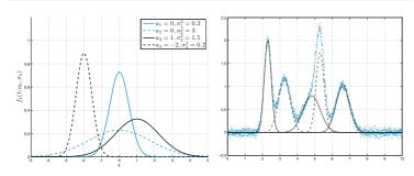
Find the set of  $(2 \times m)$  parameters that best (in the least-squares sense) represent the intensity of the recorded audio signal
