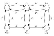
Event a (new part arrives) can only occur when the depot does not have two parts
