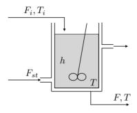
The objective of the process is to keep the liquid temperature T at target value,  $T_d$
