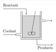
The reaction develops heat, exothermic
