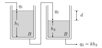
Assume that we cannot directly measure the liquid volumes in the tanks, only their difference in level. Let  $d(t) = V_1(t)/B - V_2(t)/B$  be the output variable  $(y_1(t), in control notation)$ . Also assume that the feed flow-rate from the second tank is proportional to the liquid level in that tank and that it is measured,  $q_3(t) = kV_2(t)/B$  (equivalently,  $y_2(t) = k/Bx_2(t)$ ).
