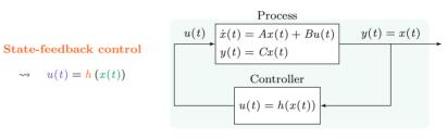
The control x(t) used to manipulate the system is a function of state x(t), we think of the controller as a device that transforms the state and feeds it back into the system
