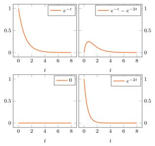
Each element of  $e^{At}$  is a linear combination of the two system modes,  $e^{-t}$  and  $e^{-2t}$
