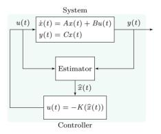
Were the state estimate  $\hat{x}(t)$  accurate, we could use it with the optimal controller (-K)
