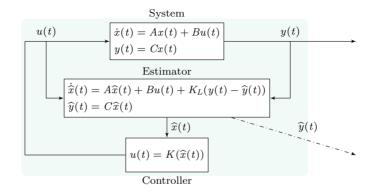
$$\begin{aligned} \dot{\hat{x}}(t) &= A\hat{x}(t) + Bu(t) + K_L y(t) - K_L \hat{y}(t) \\ &= A\hat{x}(t) + Bu(t) + K_L y(t) - C\hat{x}(t) \\ &= (A - K_L C)\hat{x}(t) + Bu(t) + K_L y(t) \\ &= \underbrace{(A - K_L C)}_{A_L} \hat{x}(t) + \underbrace{[B - K_L]}_{B_L} \begin{bmatrix} u(t) \\ y(t) \end{bmatrix} \end{aligned}$$
