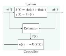
Were the state estimate  $\hat{x}(t)$  accurate, we could use it with the optimal controller (-K)
