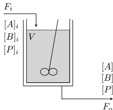
Note how the state equations of the state-space model contains also a parameter,  $k$
