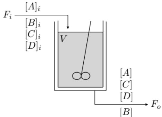
The total material balance, under the assumption of a constant volume in the tank
