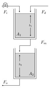
We are interested in controlling the liquid level in the two tanks and we want to use the influent flow-rate  $F_i$  to the first tank as manipulated variable. We assume that  $h_1(t)$  and  $h_2(t)$  are measured and we assume that  $F_i(t)$ ,  $F_m(t)$ ,  $F_d(t)$ , and  $F_o(t)$  are measured, too.
