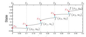
The integration of the dynamics is performed over the much sorter interval  $[t_k, t_{k+1}]$ • The forward integrator is only mildly nonlinear
