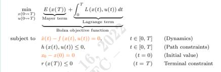
We constrain the initial value of the state to be  $x_0$ , by explicitly setting  $x(0) = x_0$ . Moreover, we constrain the state to satisfy the continuous-time dynamics in [0, T]
