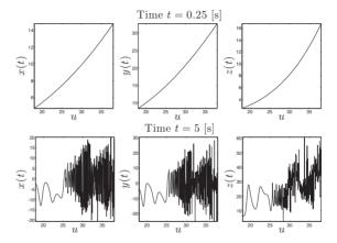
For short integration times, the relationship between states and controls is close to linear and as the becomes highly nonlinear with the duration of the simulation time
