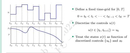
Consider the time  $t \in [t_k, t_{k+1}]$ , the zero-order hold control active on the interval is  $u_k$ .
