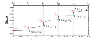
The integration over the interval  $[t_k, t_{k+1}]$  is meaningful if the shooting gap is closed
