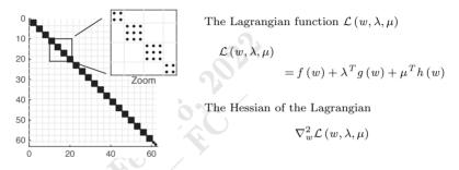
The Hessian of the Lagrangian is block-diagonal, with small symmetric blocks
