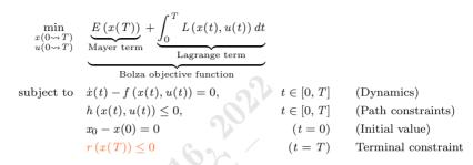
A terminal constraint is expressed as inequality constraint on the terminal state x(T)
