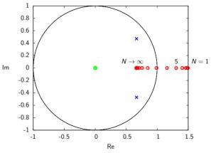
When we start with a finite horizon LQR, we move both the open-loop eigenvalues
