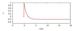
Suppose that we request a unit step of the output y(t), as a set-point change
