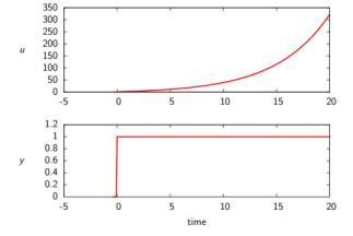
We are capable of achieving perfect tracking in y(t) by using applying an optimal u(t)
