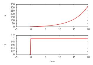
We are capable of achieving perfect tracking in y(t) by using applying an optimal u(t)
