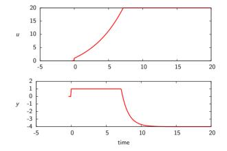
The saturation of the input at the constraint destroys the perfect output response y(t)
