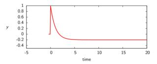
Suppose that we request a unit step of the output y(t), say a set-point change
