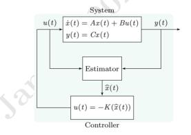
Were the state estimate  $\hat{x}(t)$  accurate, we could use it with the optimal controller (-K)
