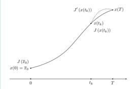
Partial optimal control trajectory
