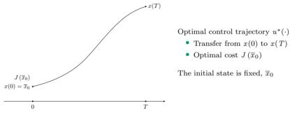
Consider a point  $t_k$  in between 0 and T, 'an optimal policy has the property that whatever the previous state and control, the remaining controls must constitute an optimal policy with respect to the state resulting from the previous decision'
