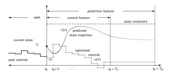
$$\min_{\substack{u_k, \dots, u_{k+N-1} \\ \forall n \in [k, k+N]}} \sum_{n=k}^{k+N-1} L(x_n, u_n) + L_f(x_{k+N})$$
