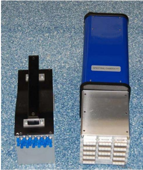
(a) Illumination unit and spectral camera
